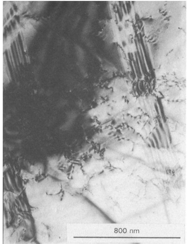
Figure 4 Transmission electron micrograph showing the austenite solidified from the molten phase. Stacking faults and dislocations are visible.
