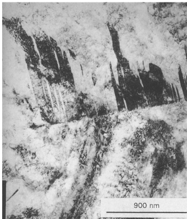
Figure 8 Transmission electron micrograph showing the twinned structure grown on the interface.
